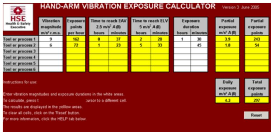
Figure 2 Screen Shot of Hand Arm Vibration Calculator
