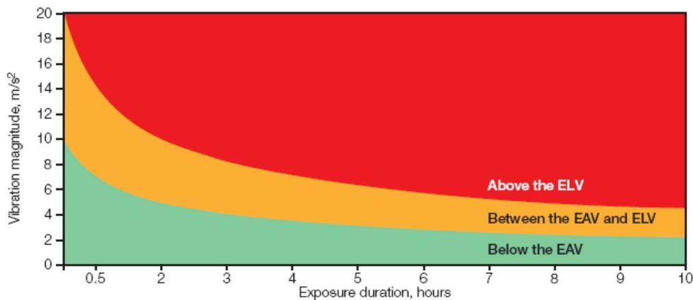
**Figure 1** How vibration level and duration affect exposure
